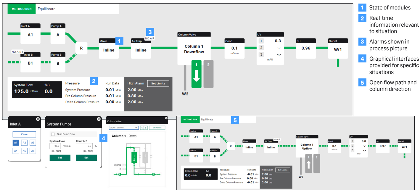
Fig 7. The process picture in UNICORN™ is interactive and only provides the necessary information at each stage. The process picture is updated to display connected modules.
