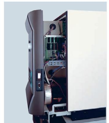
**Fast and easy service:** A service drawer ensures quick access to all electronic and heating/cooling components without the need to move or unstack the shaker.
