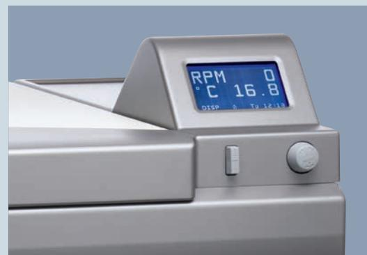
**Easy interface handling and programming:** The top-mounted controls and display make it easy to view, set and program parameters - continuous, timed, or multi-step programs with up to 15 steps (four programs storable).
