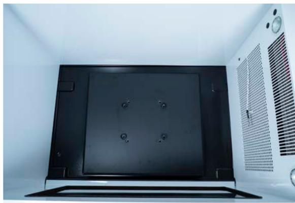
**Spill protected and easy to clean:** The drive is protected by a covering spill diverter underneath the shaker platform. It guides liquids to the drainable spill pan underneath. The spill pan can also be used as water reservoir to reduced medium evaporation – humidity monitoring is optional.
