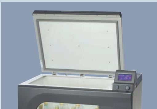
**Ergonomic design:** The easy-open lid, assisted by a foot pedal release supports smooth and safe handling even of large flasks.
