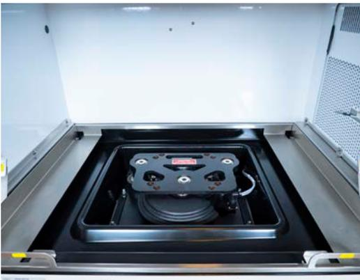
**Built to last:** The Innova triple eccentric counterbalanced drive with three weight-supporting shafts provides vibration and trouble-free operation with high loads for years. It is not to be confused with so called “triple counterbalanced” drives that usually come with only one weight support.
