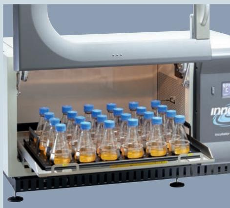
**Easy door and platform handling:** The space-saving door glides up and out of your way for easy access to all samples and easy service.
