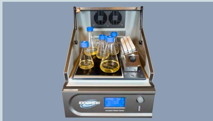
**Flexibility for various vessel formats:** The Innova 40/40R accommodates flasks up to 3L. A sticky pad platform is available for low-speed shaking (200 – 250 rpm, depending on orbit) of flat bottom vessels.
