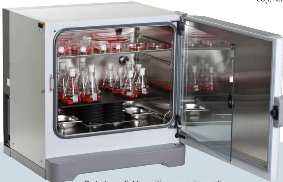
**Less noise in the lab:** One of the quietest CO<sub>2</sub> incubator shakers on the market – with the Innova triple eccentric counterbalanced drive
