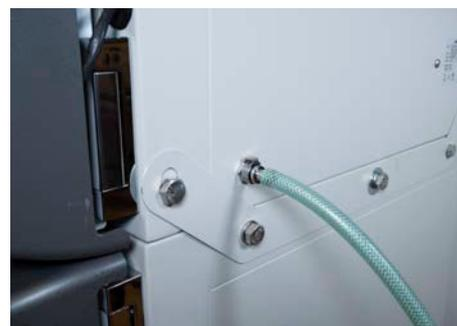
**Spill protected and easy to clean:** The Innova triple-eccentric drive is protected from spills by a covering spill diverter underneath the shaker platform (left). The spill diverter guides liquids to the drainable spill pan with rounded corners underneath (middle and right, tubing and connector not supplied). The built-in spill pan can also be used as water reservoir to reduce medium evaporation – humidity monitoring is optional.
