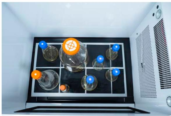
**Flexibility for various vessel formats:** The Innova 43/43R accommodates flasks up to 6 L. A sticky pad platform is available for low-speed shaking (200 – 250 rpm, depending on orbit) of flat bottom vessels.
