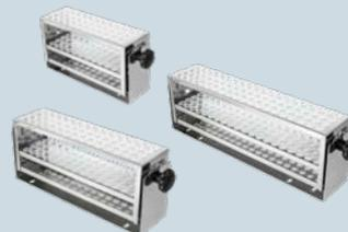
**Test tube racks** for universal platforms come in 18 formats for 8–30 mm tube diameter. The side knobs let you quickly adjust the shaking angle or release the insert rack from the holder, for easy transport to the bench. Racks come with a tube height-support, are made of stainless steel. Plastic inserts help to retain tubes and prevent them from spinning in the rack.
