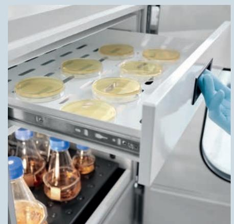
**Sample desiccation and medium evaporation protection:** The optional culture drawer can be used to protect Agar plates from desiccation. A built-in spill pan and optional humidity monitoring.
