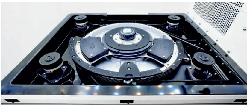
**Built to perform and last – the patented Eppendorf X-Drive:** With its five eccentric mounting points for the shaker platform, the drive is precisely engineered to ensure long-lasting, repeatable performance with high loads over years. The four shafts in the corners and Balance Master Technology support precise vibration-free shaking on every point of the platform, including the periphery.
